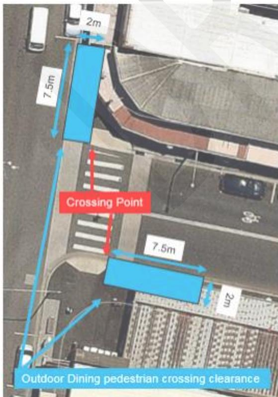
Figure 3: Minimum pedestrian crossing clearances when approaching a signalised pedestrian crossing
