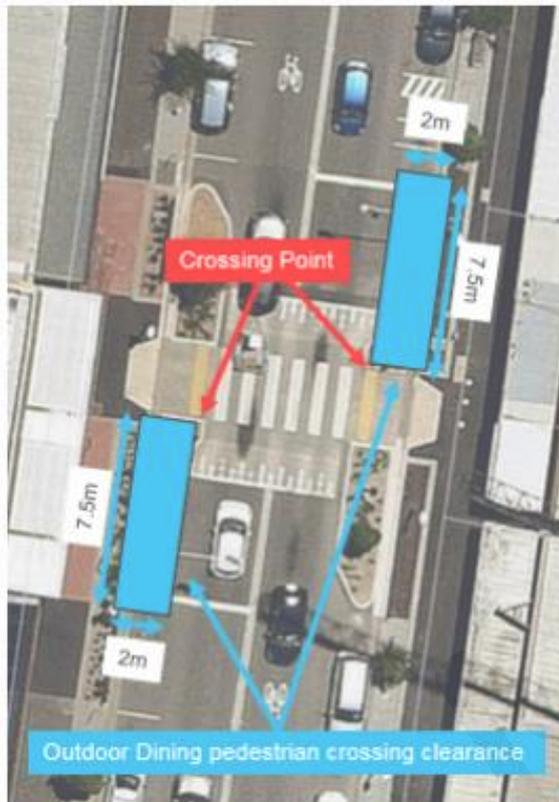
Figure 2: Minimum pedestrian crossing clearances when approaching an unsignalled/ zebra pedestrian crossing without a kerb extension.
